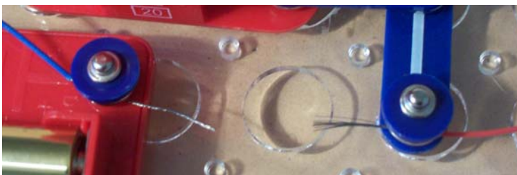
Image 1: Connecting wires into a Brainbox circuit using the single press stud connectors.
