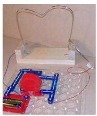
This circuit can be added into a *BrainBox* sound module or lighting circuit replacing the normal switch. The wire shape was made from a coat hanger and several pieces of wood. Wires are connected as in the photo and then snapped into the *BrainBox* circuit (I used the design on page 8 – be warned you get sick of 'Happy Birthday' after a while).
